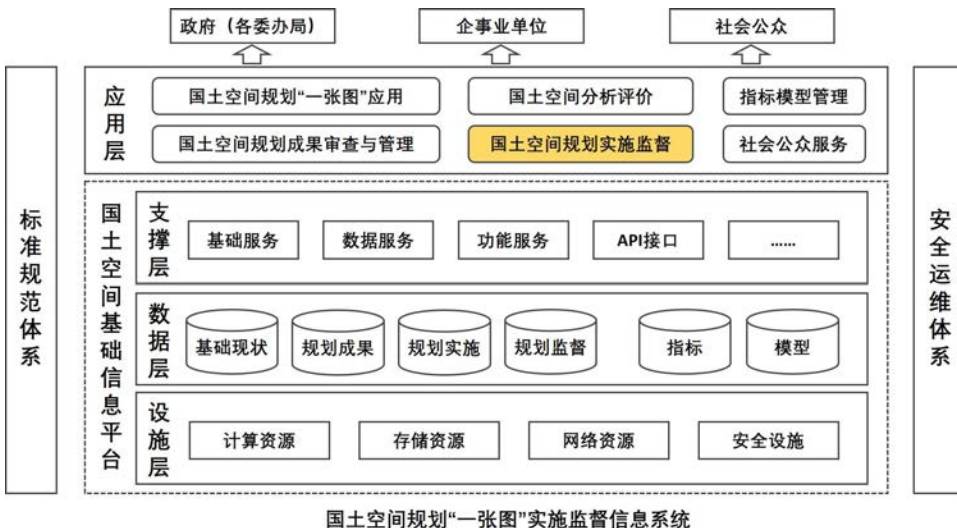
图1 国土空间规划实施监督子系统和国土空间规划“一张图”实施监督信息系统关系示意图 Fig.1 The relationship between the implementation and supervision of spatial planning subsystem and the 'Inteplan' information system for implementation and supervision of spatial planning
