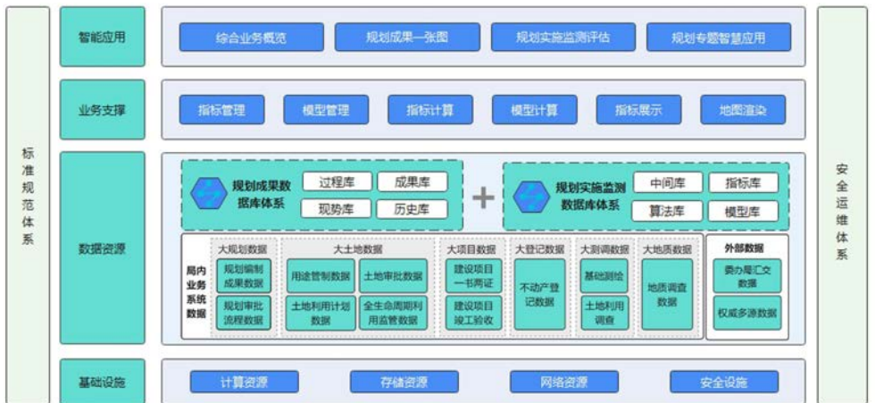
图3 上海市规划驾驶舱系统架构 Fig.3 The framework of the cockpit of spatial planning for Shanghai
