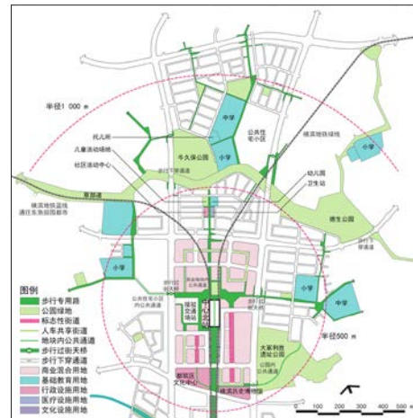
图6 港北新城中心北站TOD地区的步行专用路网络 Fig.6 Pedestrian network in the TOD area of Central North Station in Kohoku New Town 资料来源:根据参考文献[37]9, [38]8-9改绘。
