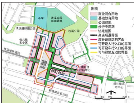
图8 港北新城仲町台站前街区营造协定引导图则 Fig.8 Guidelines of the construction agreement for the Nakamachidai Station Core Area in Kohoku New Town
