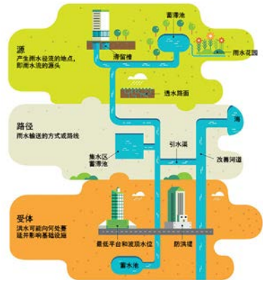
图4 新加坡的雨水管理系统 Fig.4 Stormwater management systems in Singapore 资料来源: Singapore's National Water Agency (PUB)官网 https://www.pub.gov.sg/ 。
