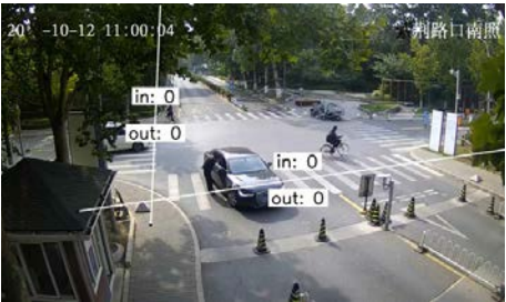
图4 使用YOLOv8、ByteTrack和Supervision进行骑手检测、跟踪和计数 Fig.4 Using YOLOv8, ByteTrack and Supervision for rider detection, tracking and counting
